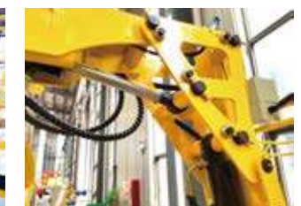
Folding arm and hydraulic cylinder
