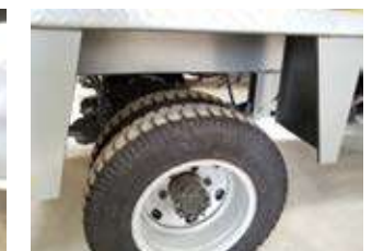
Rear four wheels and steel plate suspension
